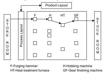
Fig. 2.7 Combination layout for making different types and sizes of gears
