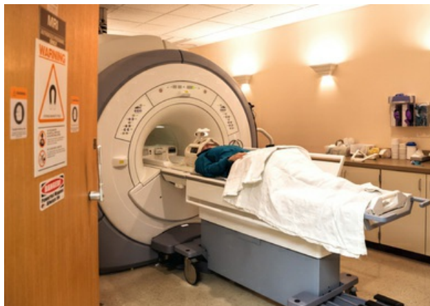
FIGURE 2-10 Patient entering an MRI unit surrounded by a superconducting 1.5-Tesla magnet. Magnetic field changes are picked up by the surrounding machine and processed by a computer to create images. For this examination, the patient must lie very still and have no metal objects on or within the body. (Courtesy GE Medical Systems, Milwaukee, Wisconsin.)
